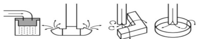
Figure 7 Examples of calming inlets
